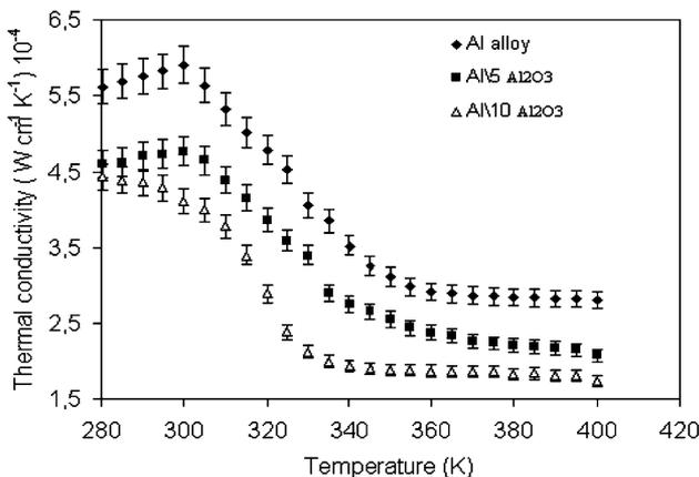
**Fig. 8** The effect of the Al<sub>2</sub>O<sub>3p</sub> particulates on the thermal conductivity of Al\Al<sub>2</sub>O<sub>3</sub> MMCs
