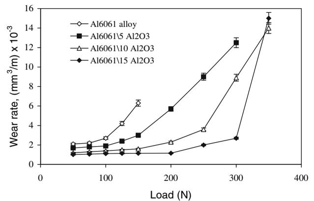
**Fig. 5** The effect of load on wear rate of Al6061 alloy and Al6061/Al<sub>2</sub>O<sub>3</sub> MMCs (Ambient temperature)
