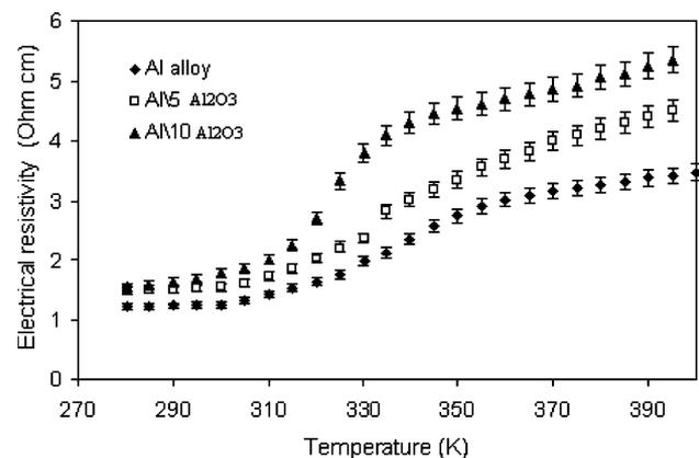
**Fig. 7** The effect of the Al<sub>2</sub>O<sub>3p</sub> particulates on the electrical resistivity of Al/Al<sub>2</sub>O<sub>3</sub> MMCs
