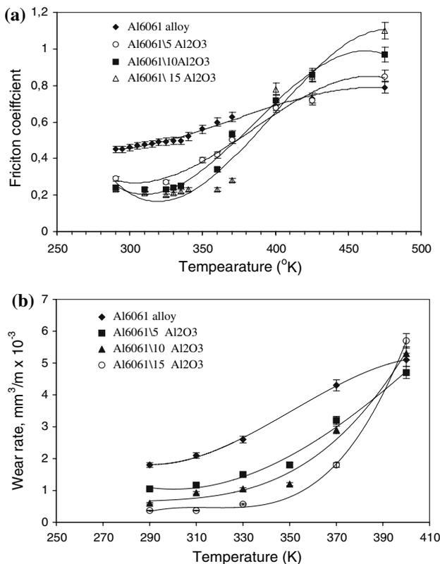
**Fig. 6** (a) The effect of the temperature on the friction coefficient, (b) The effect of the temperature on wear rate under an external supplied heat (80 N)
