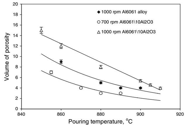
**Fig. 2** The effect of pouring temperature on porosity content of Al6061 alloy and Al6061/10 vol% Al<sub>2</sub>O<sub>3</sub> MMCs
