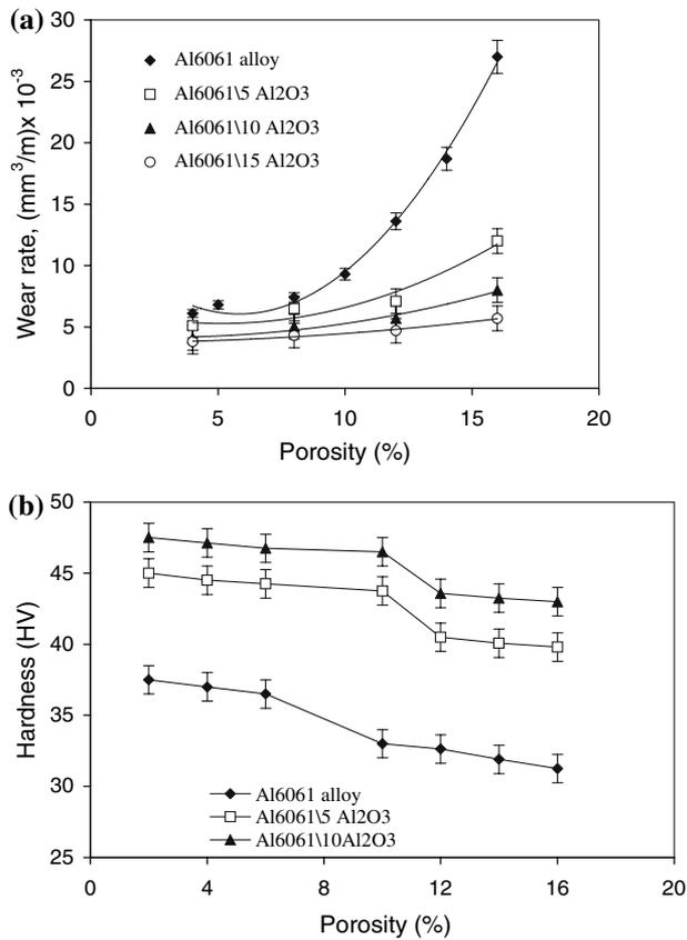
**Fig. 3** (a) The effect of porosity on wear rate of Al6061 alloy and Al6061/Al<sub>2</sub>O<sub>3</sub> MMCs at ambient temperature, (b) The effect of porosity on hardness of Al6061 alloy and Al6061/Al<sub>2</sub>O<sub>3</sub> MMCs
