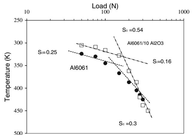
**Fig. 9** The change of the contact surface temperatures of the worn surfaces of Al6061 alloy and Al6061/10 vol% Al<sub>2</sub>O<sub>3</sub> MMCs after sliding to 1,000 m vs. load during dry sliding at ambient temperature. (S<sub>I</sub> = Slope of temperature change before transition temperature, S<sub>II</sub> = Slope of temperature change after transition temperature)
