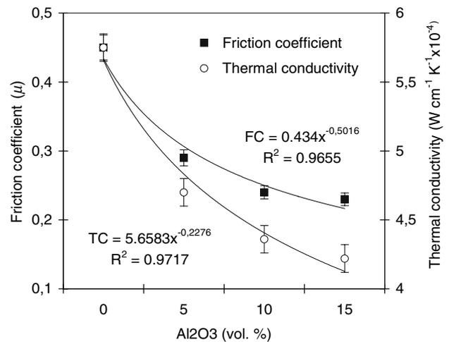
**Fig. 10** The effect of Al<sub>2</sub>O<sub>3p</sub> particulates on the friction coefficient and the thermal conductivity at 290 K temperature
