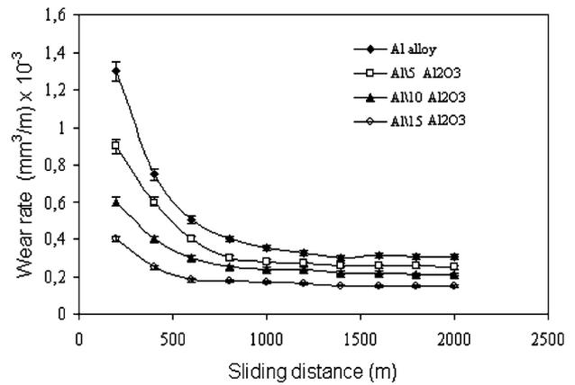
**Fig. 4** The effect of sliding distance on wear rate of Al6061 alloy and Al6061/Al<sub>2</sub>O<sub>3</sub> MMCs at ambient temperature
